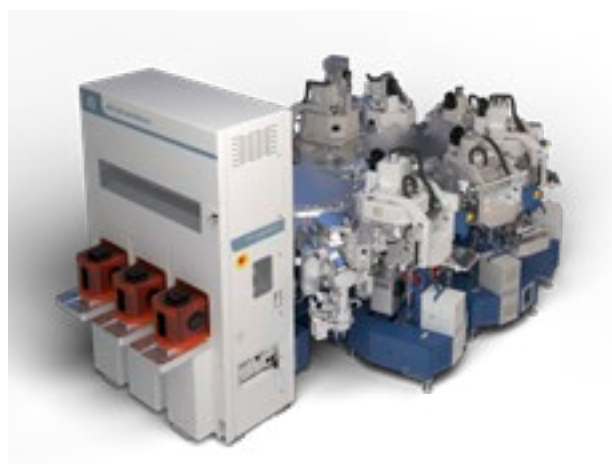
Figure 2. The Endura® Impulse™ PVD platform for PCRAM and ReRAM includes up to nine process chambers integrated under vacuum along with on-board metrology.
