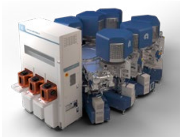
Figure 1. The Endura® Clover™ MRAM PVD platform is made up of nine unique wafer processing chambers all integrated in pristine, high-vacuum conditions.
