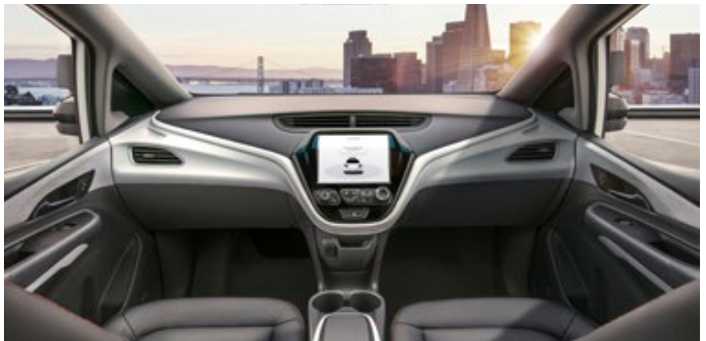
Chevy Bolt Cruise AV test vehicle on display this week doesn't have a steering wheel
