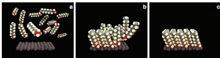
FIGURE 3. Schematic Depiction of SAM Formation of a Monolayer-thick Film.
