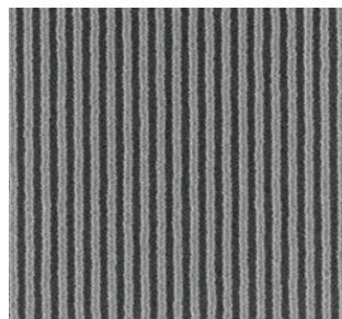
FIGURE 5. Dense line spaces patterned at pitch 40nm.
