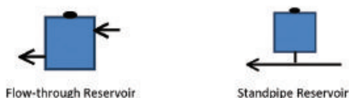
FIGURE 1. The reservoir can be designed as a flow through reservoir or as a standpipe reservoir with a pressurized cap.
