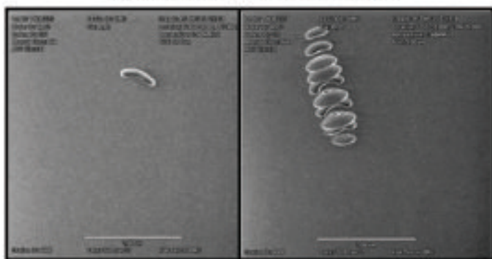
FIGURE 4. Normalized scratch defect comparison on USG wafers and examples of scratch defects.
