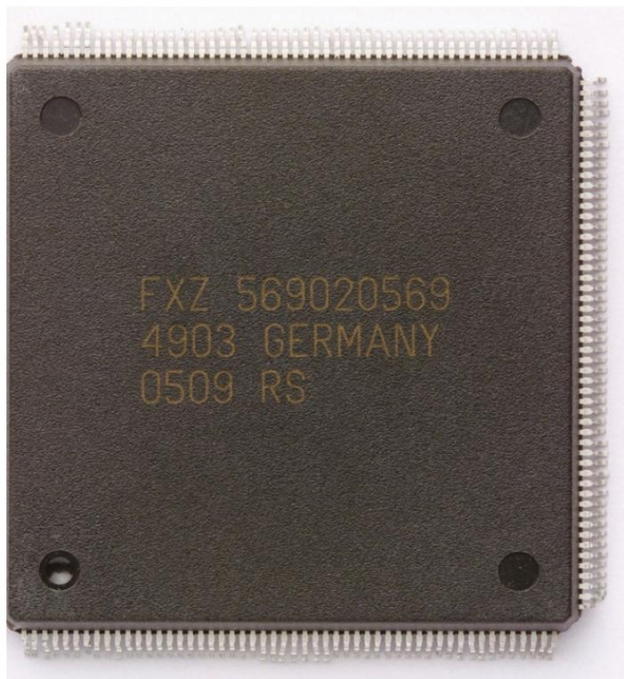
**FIGURE 2.** Standard thickness molded IC package marked with 30 W, near IR DPSS laser (PL E Air 30 D IC).
