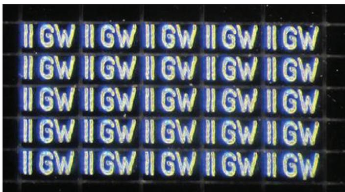
**FIGURE 5. c)** backside of silicon wafer marked with characters <math>< 150 \mu\text{m}</math> in height
