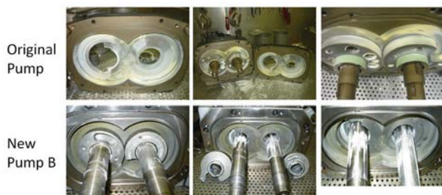
FIGURE 7. Pictures comparing the third stage of the original pump and New Pump B showing the different deposition patterns.
