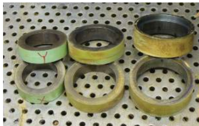
FIGURE 6. Picture of sleeves in an exchanged pump showing deposition on the outer surfaces.
