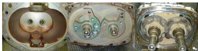
FIGURE 2. Pictures of a disassembled pump that was removed for inspection after only 457 hours due to a large current spike detected during operation. In order, the pictures show the booster, second stage of the dry pump, and the final stage of the dry pump.
