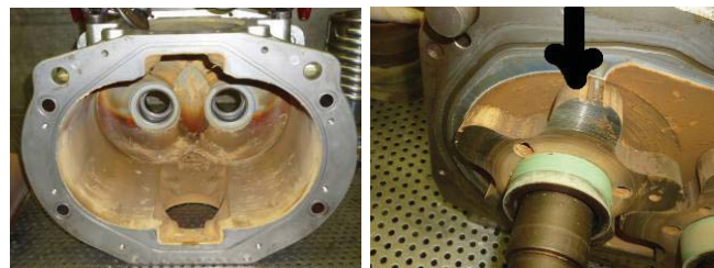
FIGURE 1. A picture of a disassembled pump after 1,200 hours of use on a high-k ALD process showing the deposition in the booster (left) and loss of clearance in the last stage of the dry pump (right).
