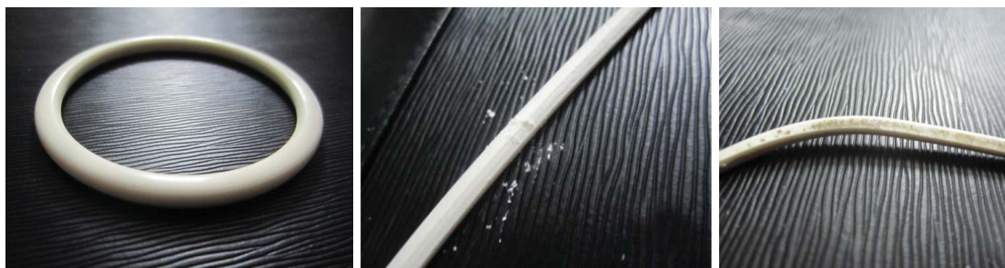
FIGURE 1. Seal failures can be caused by compression (left), powdery contamination from etching (middle), or damage due to poor installation (right).
