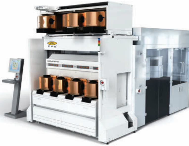
FIGURE 4. The EVG GeminiFB fusion wafer bonding system integrates wafer cleaning, LowTemp ® plasma activation, SmartView ® wafer-to-wafer alignment system and wafer bonding all in one system.
