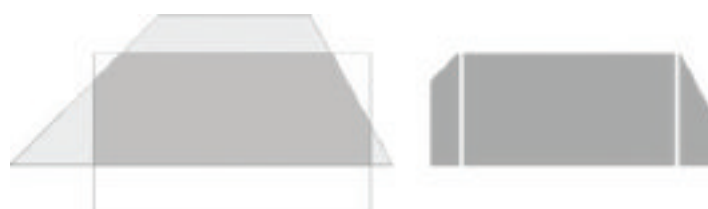
FIGURE 5. Clipping a trapezoid with a rectangular area will always generate a convex polygon that can be fractured in never more than 3 trapezoids.
