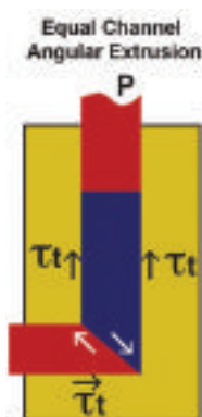
FIGURE 1. Schematic of ECAE (note: P is punch pressure and \tau_t is the friction along channels) and conventional TMP.
