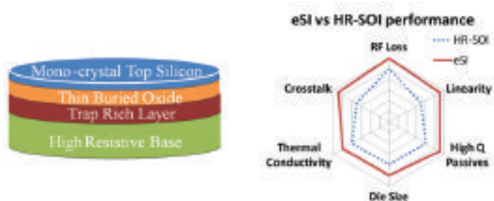
FIGURE 13. Gen 2 HR-SOI (eSi) substrates, advantages vs Gen 1 HR-SOI substrate.
