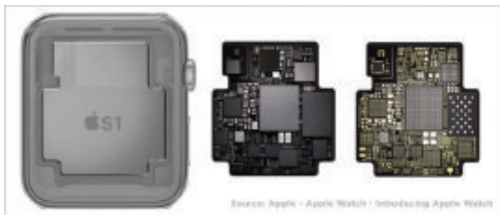
FIGURE 2. Compact integration of multiple chip and sensor technologies for IoT devices will demand more sophisticated system- in-package technology. The new Apple Watch has 30 components in its core S1 SiP, all packed on to a 26mm x 28mm motherboard and overmolded with a conventional IC packaging resin compound. (Source: Chipworks)
