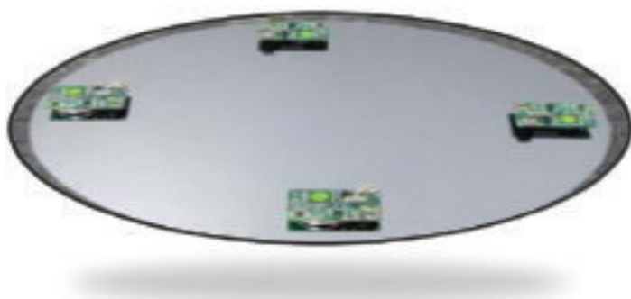
FIGURE 3. Silicon Wafer With 4 RH Recording Sensors Taped on.
