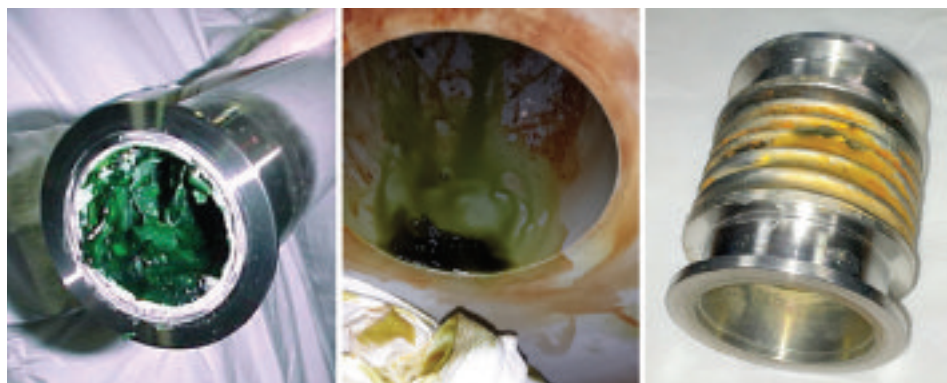
FIGURE 2. (left) Acidic TEOS-based polymer with a pH of approximately 1, (middle) Condensed corrosive Br 2 -based liquid, (right) Exhaust pipe damaged by exposure to condensed acidic material.
