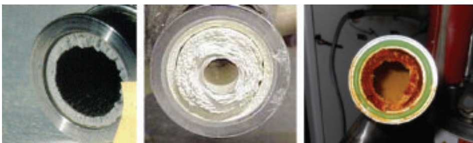
FIGURE 3. Exhaust blockage caused by various materials (left) AlCl 3 from a metal etch process, (middle) NH 4 Cl from an LPCVD process, (right) Unknown material deposited in the exhaust of a metal carbide CVD process.
