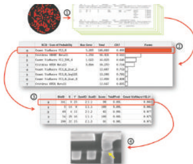
FIGURE 1. Typical application: Root Cause Deconvolution determines root cause distribution and devices most likely to fail for each root cause. Defect courtesy [2].
