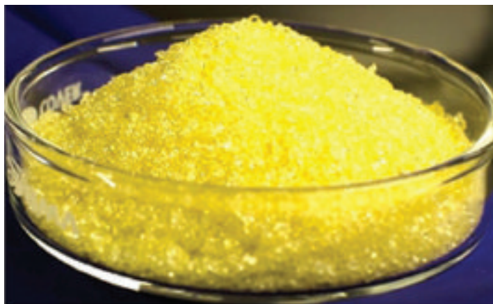
FIGURE 1. Improved methods of purification have been used to produce microcrystalline pale yellow PDMAT with purity of >99.99995% (determined by trace metals and other spectroscopic methods) with extremely low chloride (<10ppm), low oxygen and total trace metals.
