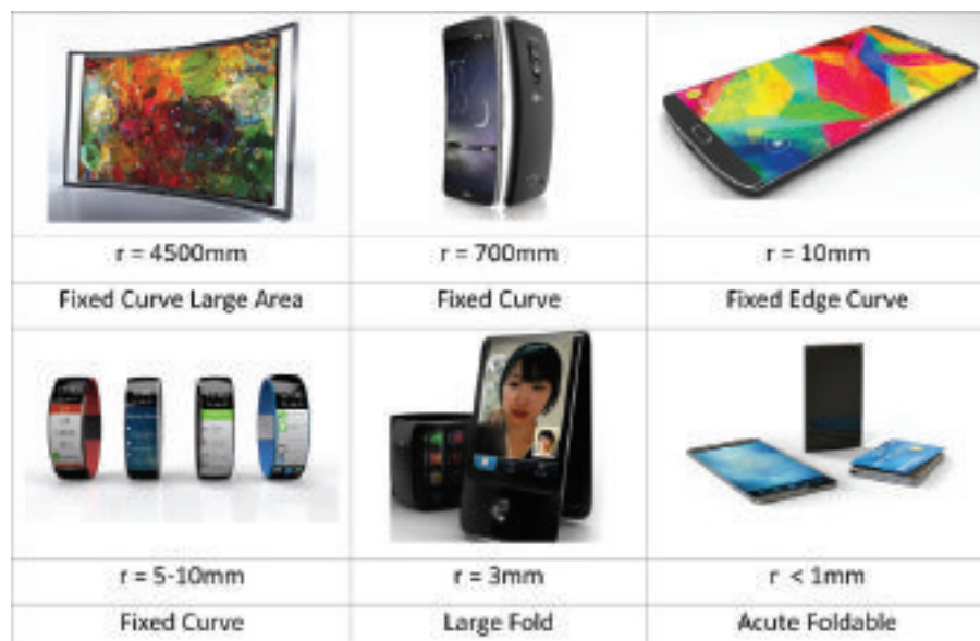
FIGURE 2: Display form factor dependency on bend radius.
