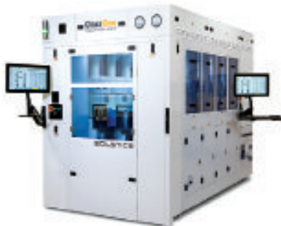
Solstice S8 for cassette-to-cassette automated plating
