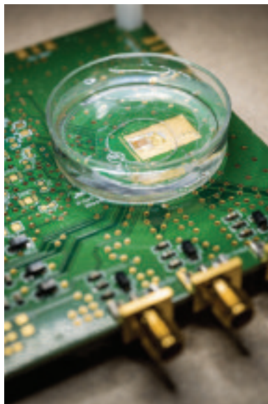
FIGURE 1. A CMOS multi-modality cellular sensor array chip being developed at Georgia Tech is hosted on a standard printed circuit board (PCB) and is packaged using low-cost polydimethylsiloxane (PDMS) material to ensure biocompatibility and electrical insulation. A standard 35 mm cell culture dish with drilled-out bottom is mounted on the PCB to host the cells and medium, and expose cells to the CMOS sensing surface. (Georgia Tech Photo: Rob Felt)
