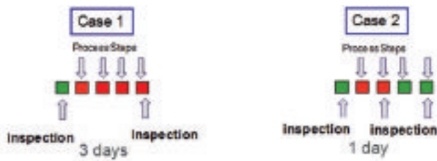
FIGURE 4. Adding an additional inspection point to the line will reduce the material at risk should an excursion occur after the first process step.
