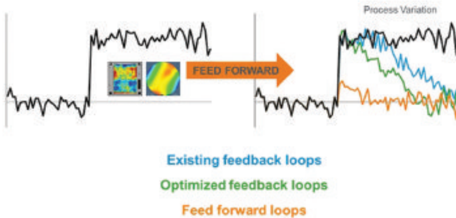
FIGURE 3. Multiple data loops to help optimize fab-wide processes. Existing feedback loops (blue) have existed for several design nodes and detect and compensate for process variations. New, optimized feedback loops (green) provide earlier detection of process changes. Innovative feed forward loops (orange) utilize metrology systems to measure variations at the source, then feed that data forward to subsequent process steps.
