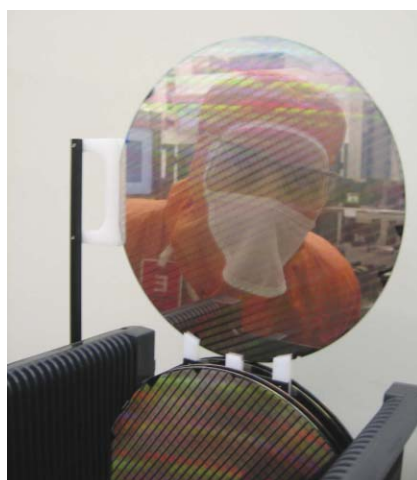
FIGURE 1. Manually inspecting a wafer on an H-bar tool.
