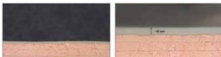
FIGURE 4. Cross section showing plated Cu with bright Ni smoothing layer to decrease surface scattering.
