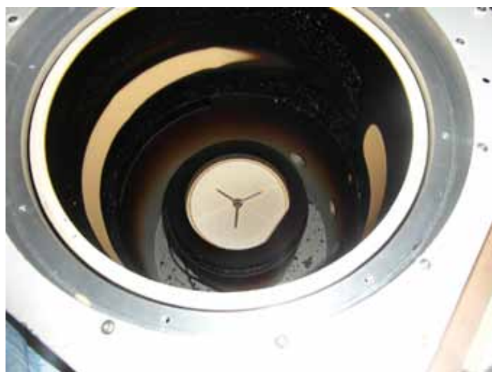
FIGURE 1. Typical chamber condition of a system which has failed for polymer defects detected on product post-processing.
