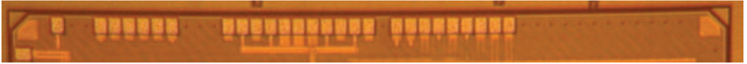
FIGURE 1. In this image, the bonding pads are grouped in tight clusters rather than evenly distributed across the edge of the chip. This makes it harder to bond to the pads and requires more-precise equipment to do the bonding, thus unnecessarily increasing the assembly cost and potentially impacting device reliability.
