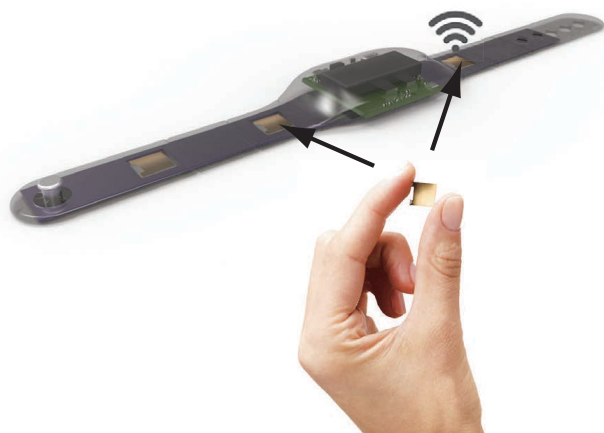
FIGURE 1. Novasentis (Burlingame, Calif.) is integrating its electro-mechanical polymer (EMP) actuator technology into wearable devices to enable real-time haptic feedback. (Photo courtesy Novasentis)
