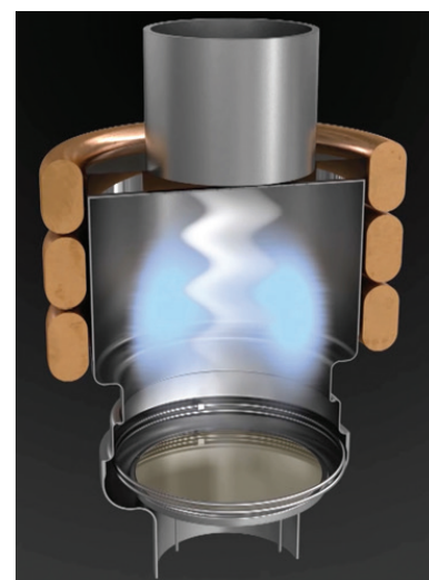
FIGURE. Cross-sectional schematic of a new Microwave Electron Cyclotron Resonance (MECR) plasma source from Hitachi High-Technologies connected to a single-wafer Atomic Layer Deposition (ALD) processing chamber from Picosun. (Source: Picosun)
