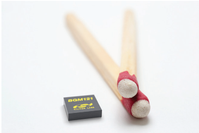
FIGURE 1. System-in-package (SiP) solutions ease the design cycle for engineers using Bluetooth and low-power wireless networks. (Source: Silicon Laboratories).
