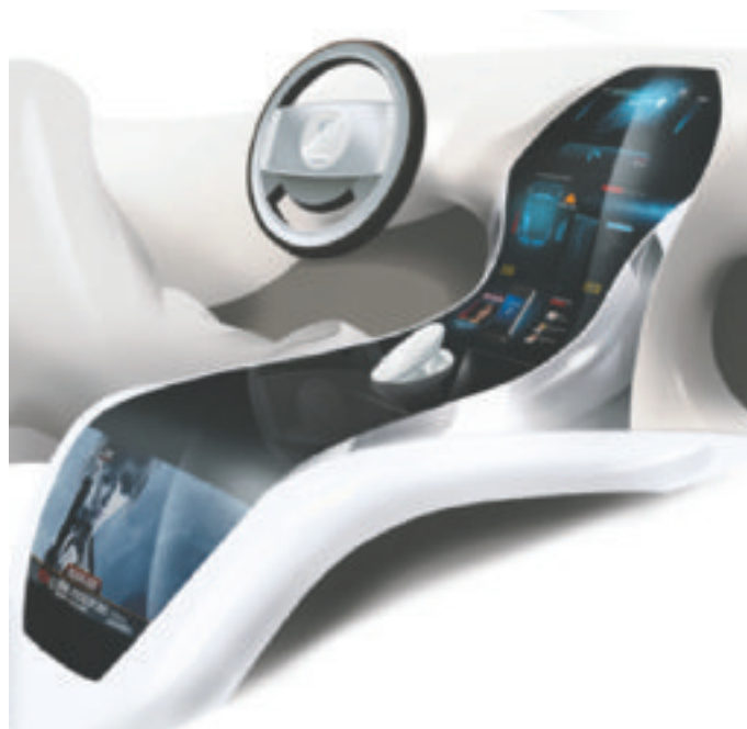
FIGURE 4. Atmel's XSense sensors can be used on curved surfaces and edges, facilitating the design of futuristic in-vehicle touchscreens and surfaces.
