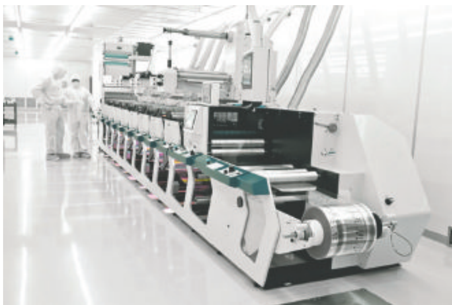
FIGURE 1. Roll to Roll Micro-contact printing line (Source: UniPixel)
