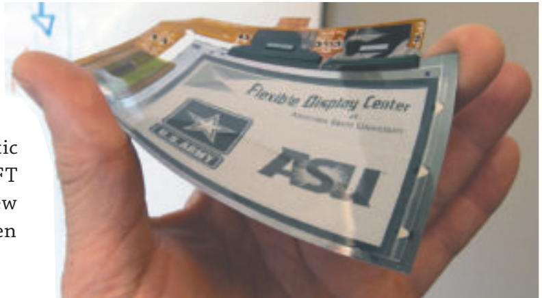
FIGURE 3. A flexible display manufactured at the Arizona State University Flexible Center. The center is unique among the U.S. Army's University centers, having been formed through a 10-year cooperative agreement with Arizona State University in 2004.
