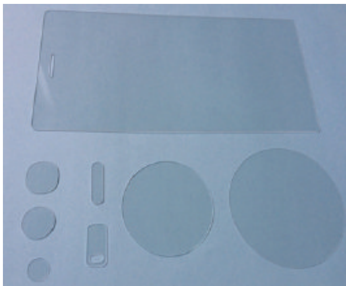
FIGURE 2. Mobile device sapphire parts partway through their production process. Figure courtesy of Chitwing-Silian.
