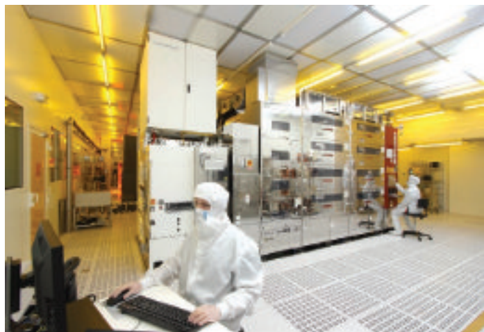
FIGURE 7. MAPPER FLX-1200 in Leti cleanroom interfaced with a SCREEN DUO track. Key figures of the tool: Acceleration voltage 5kV; throughput: 1wph with 1,300 beamlines; resolution/alignment specs: 32nmhp / 10nm 3 \sigma .
