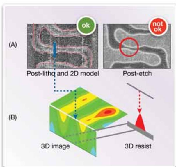
**FIGURE 2.** “Weak lithography spot” often becomes only visible after etch if 2D models are used for correction and verification.
