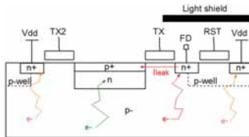
**FIGURE 3.** cross-section of a 5T charge domain global shutter pixel
