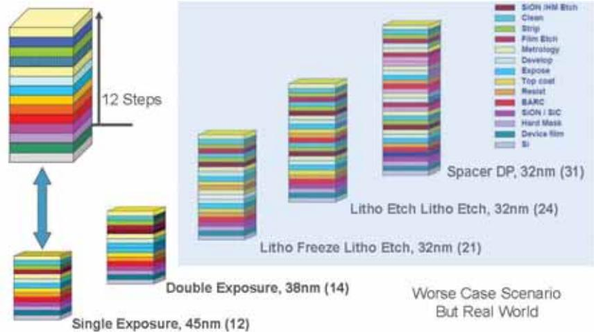
**FIGURE 2.** Multi-patterning adds many process steps, and cost. Source: ASML.
