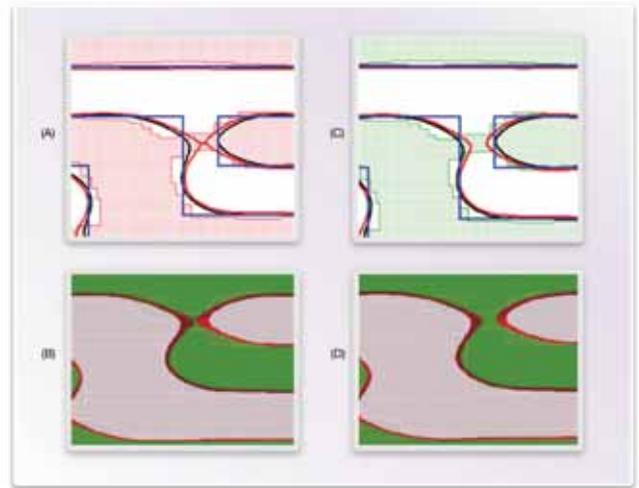
**FIGURE 5.** Successful OPC correction of an ILT mask, based on 3D resist compact model input.
