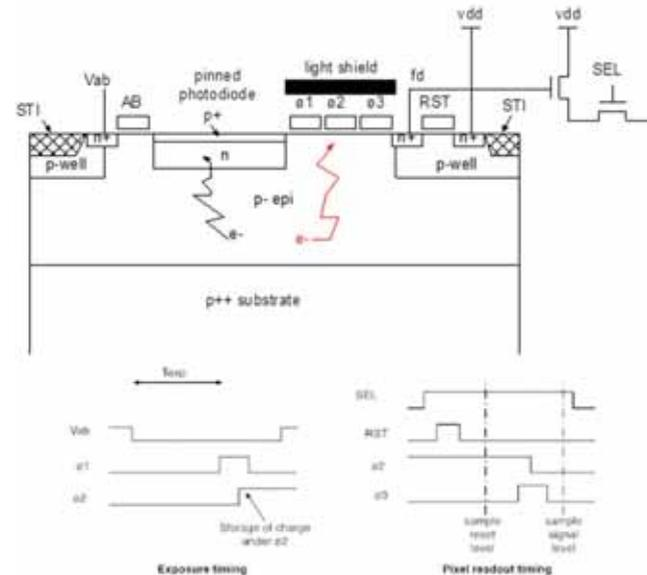
**FIGURE 4.** CDS charge domain global shutter pixel and timing
