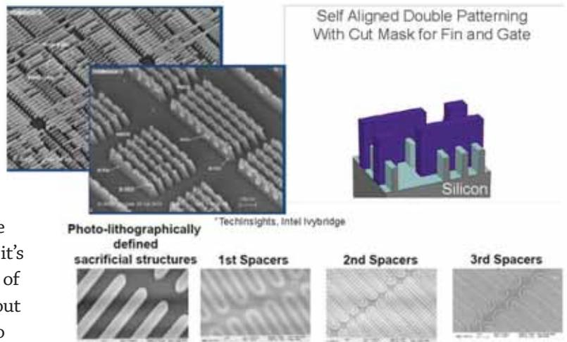
**FIGURE 1.** Multi-patterning can achieve sub-10nm dimensions. Source: Applied Materials.
