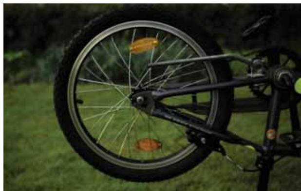
**FIGURE 1.** Rolling shutter image artifacts in the spokes of the turning wheel
