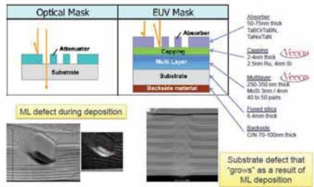
**FIGURE 3.** EUV masks are considerably more complicated than conventional photomasks. Source: Veeco.
