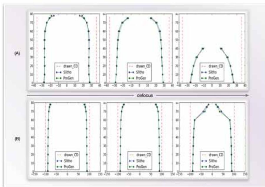
**FIGURE 4.** Rigorously tuned 3D resist compact models can predict the impact of process variation on profiles without additional data fitting.
