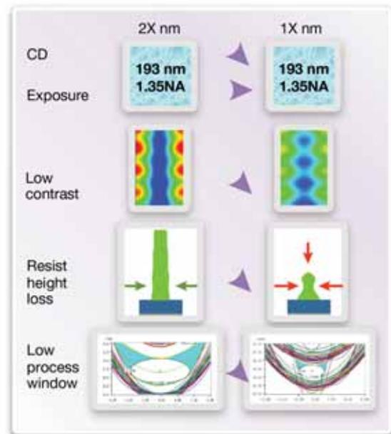
**FIGURE 1.** Extending 193nm immersion technology to the 1x technology node reveals new patterning challenges.
