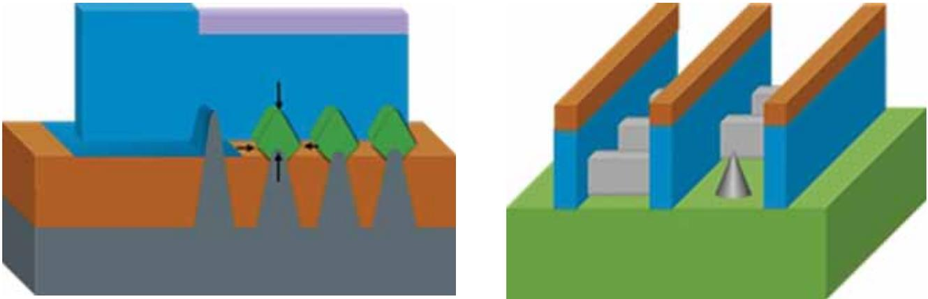
**FIGURE 1.** You can't fix what you can't find. And you can't control what you can't measure. Left: P-MOS SiGe critical dimension measurement. Right: Fin patterning particle leading to a Fin Spire defect at post dummy gate etch. Source: KLA-Tencor
