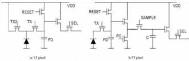
**FIGURE 2.** 5-transistor charge domain global shutter pixel (a) and 7-transistor charge domain global shutter pixel (b).
