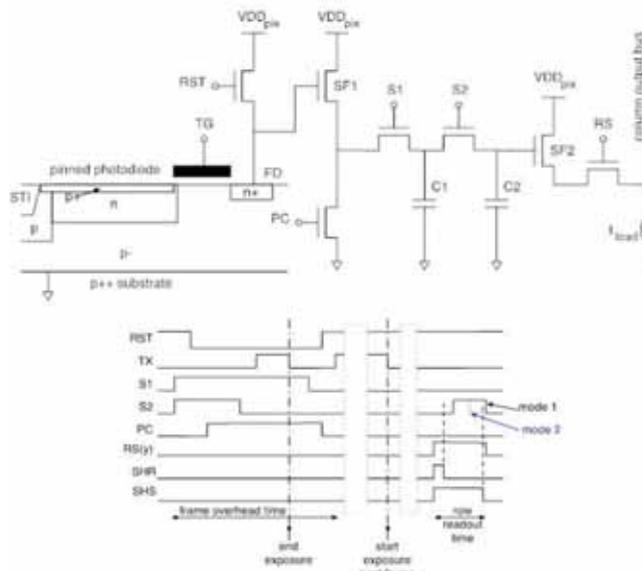
**FIGURE 5.** Voltage domain global shutter pixel with CDS
