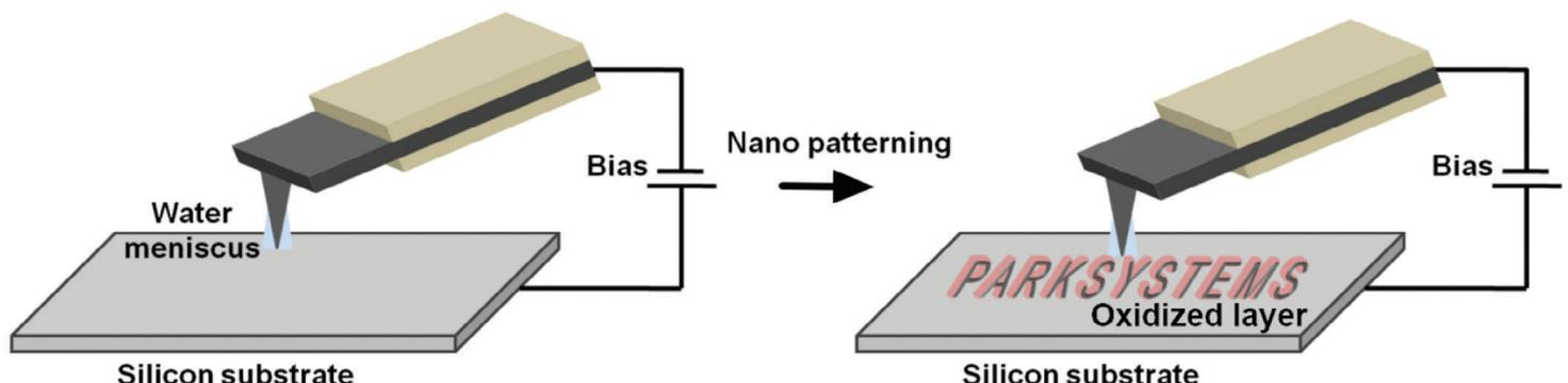
**Figure 1.** Schematic representation of bias-assisted AFM nanolithography via local surface oxidation. Patterns are created on the surface by oxidation upon bias application between tip and sample.
