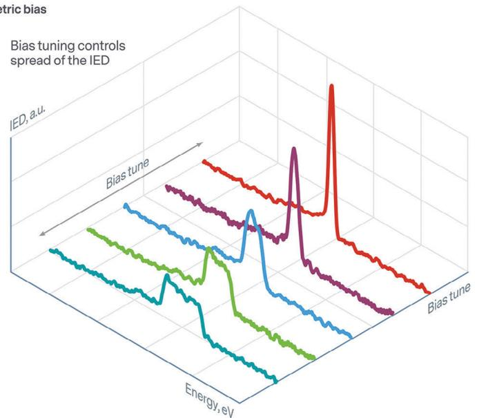
**Figure 8.** The AE eVoS non-RF, asymmetric bias system [3] allows independent setting of bias magnitude and bias tuning, separating controls of IED average from IED width [4].
