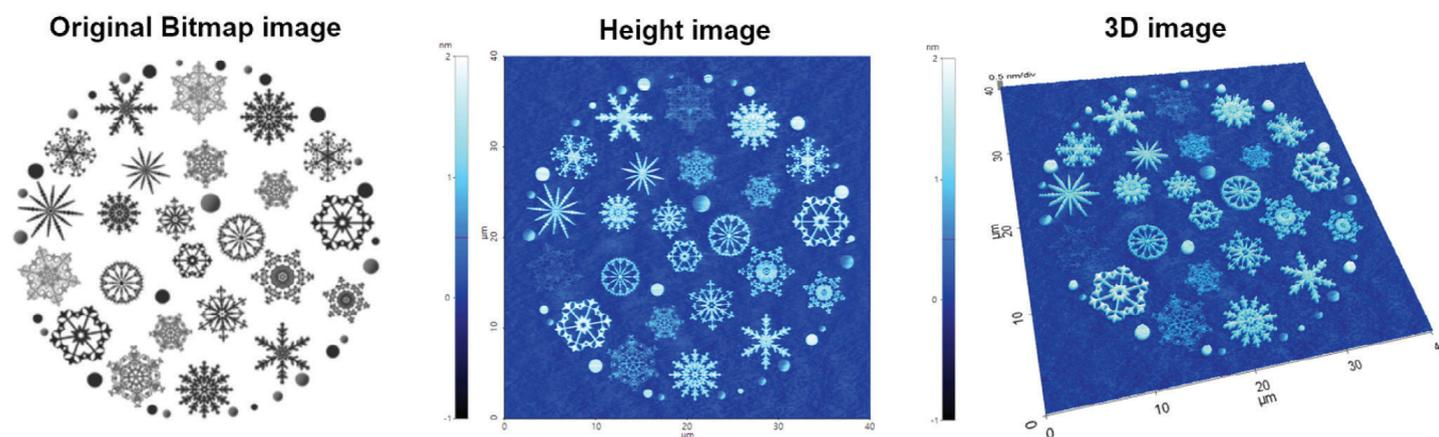
**Figure 3.** Original bitmap image used as the template (left), AFM height image after bias assisted AFM nanolithography (center) and corresponding 3D image of the sample surface (right). The nanopatterning was generated by surface oxidation.
