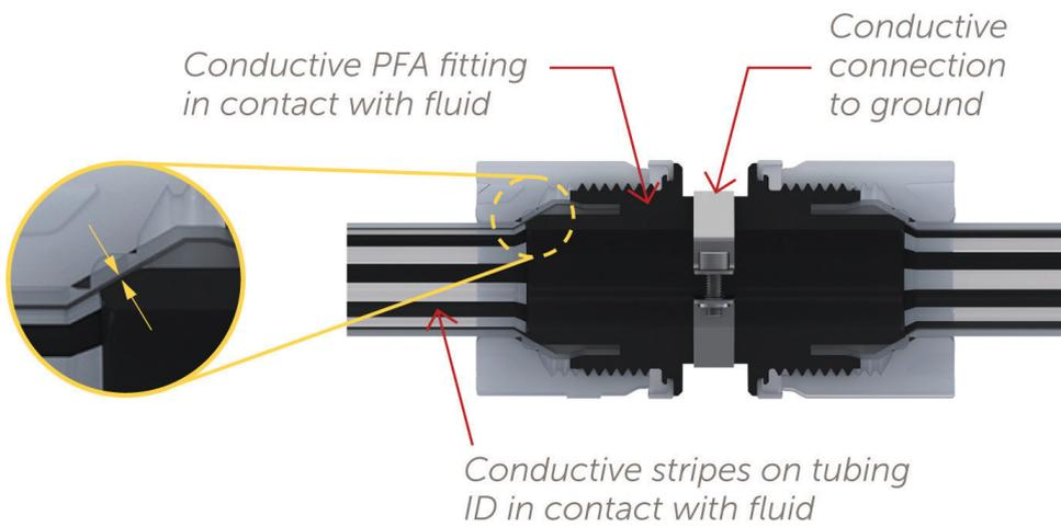
**Figure 4.** Conductive tubing with stripes on ID and carbon-loaded fitting to facilitate ground.
