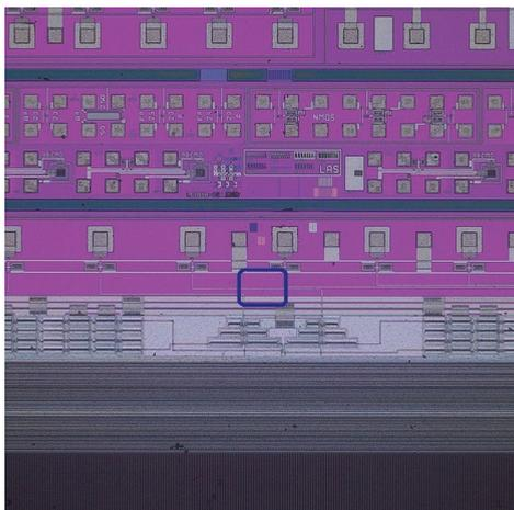
**Figure 2.** Brightfield observation: Defect detection at low magnification (70X).
