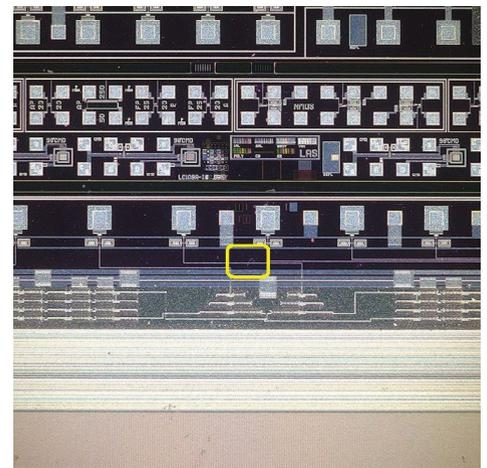
**Figure 3.** Darkfield observation: Defect detection at low magnification (70X).
