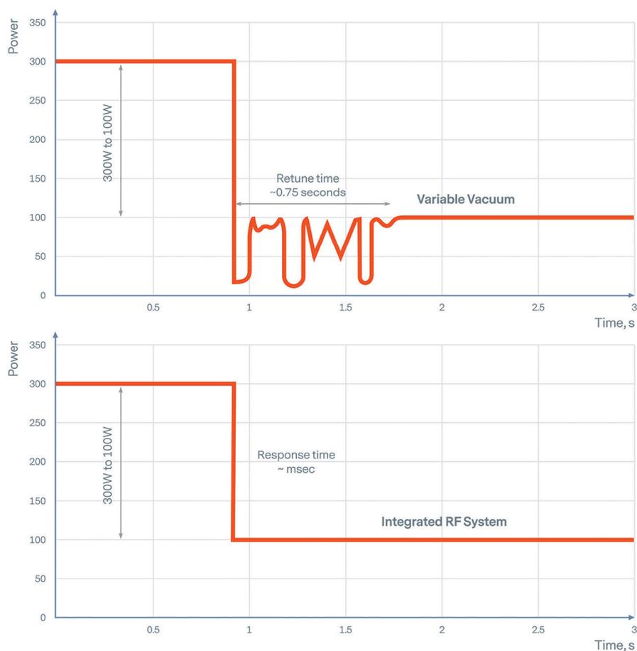
**Figure 3.** Shown is an integrated RF system delivering power to a setpoint change from 300W to 100W within a millisecond timeframe compared with typical vacuum capacitor matching network tune times of a second or more. This ensures constant, repeatable power delivery where the near-instant tuning increases productivity for these very short, high-cycle count plasma Deposition processes.
