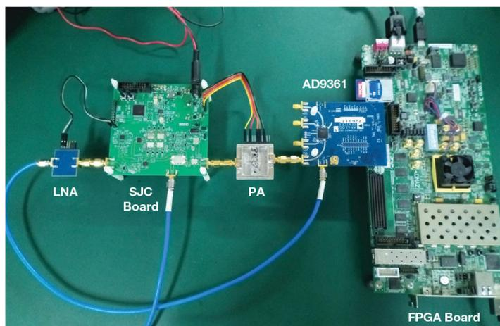
**Figure 10.** Test setup photo.
