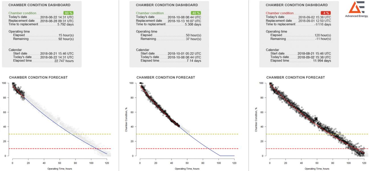
**Figure 11.** 11a: chamber in good condition. The blue line indicates the predictive chamber condition based on ingested data. 11b: chamber still in good condition, the model blue line adjusts the prediction based on usage and more ingested data. Notice slope of line has changed. 11c: chamber must be serviced as the threshold for maintenance has been crossed (red line). The yellow line indicates an earlier warning which can be set by the customer.
