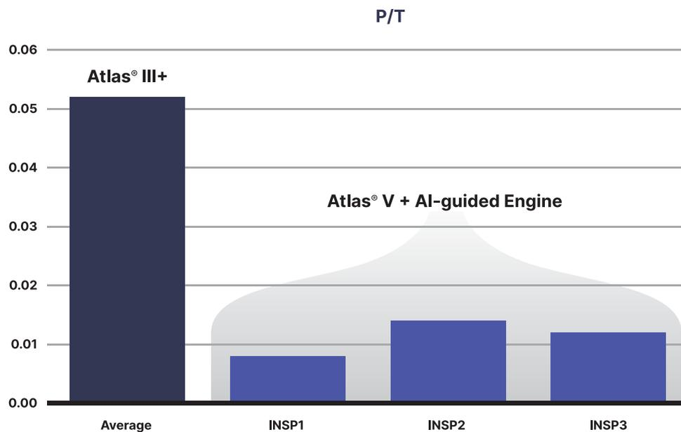
**Figure 5.** One of the greatest metrology challenges in the GAA process flow is the measurement of inner spacer cavity etch and the inner spacer itself. The latest generation systems can provide individual spacer measurements with several times better precision/tolerance than the average measurements available from previous generation systems.
