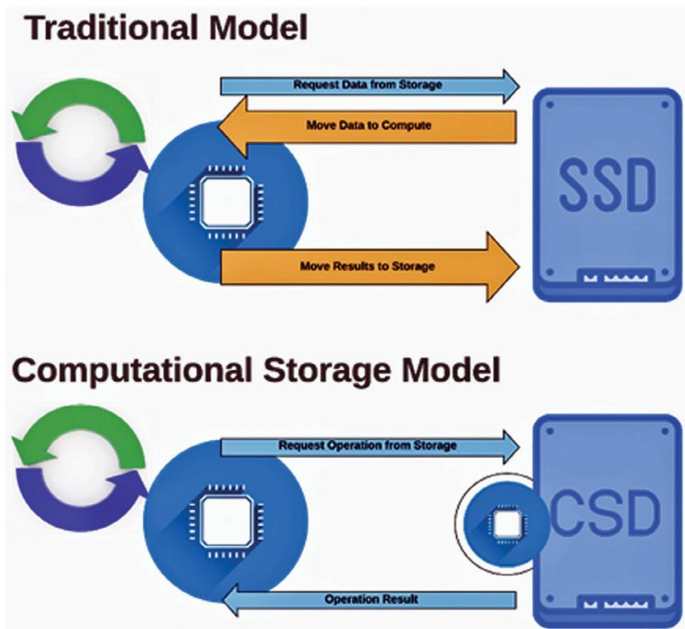
**Figure 1.** CSD eliminates data transfers with the host computer by performing computations locally within the SSD.
