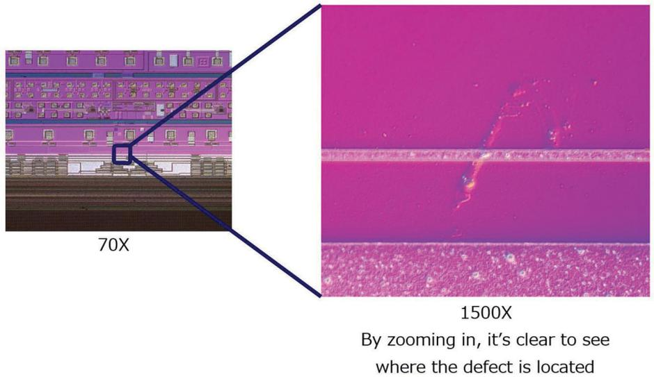
Figure 5. Defect viewed at 1500x under DIC observation
