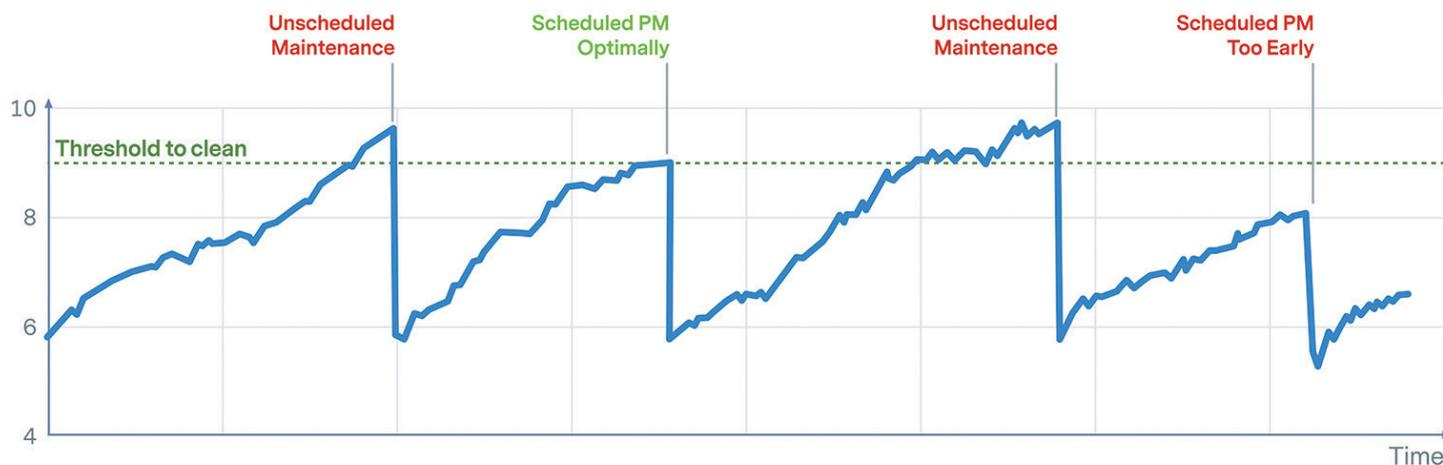
**Figure 9.** Time-based preventive maintenance cycle indicates non-optimized maintenance cycles. Green dashed line indicates optimal condition for PM.
