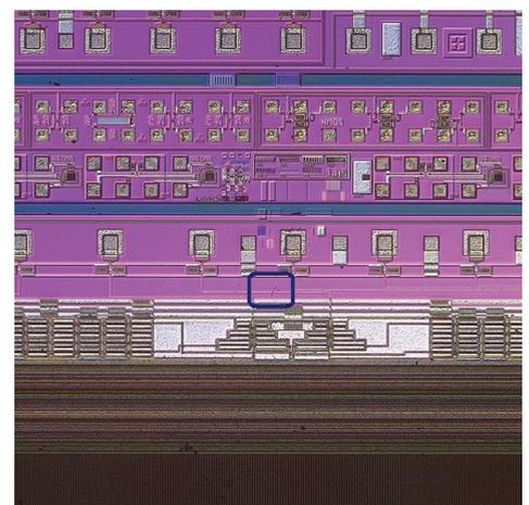
**Figure 4.** DIC observation: Defect detection at low magnification (70X).
