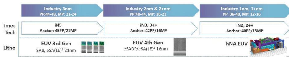
**Figure 1.** An imec view on the EUV lithography roadmap (PP=poly pitch; MP=metal pitch; SAB=self aligned blocks; eSALELE=innovative approach to self-aligned litho-etch litho-etch; SADP=self-aligned double patterning).
