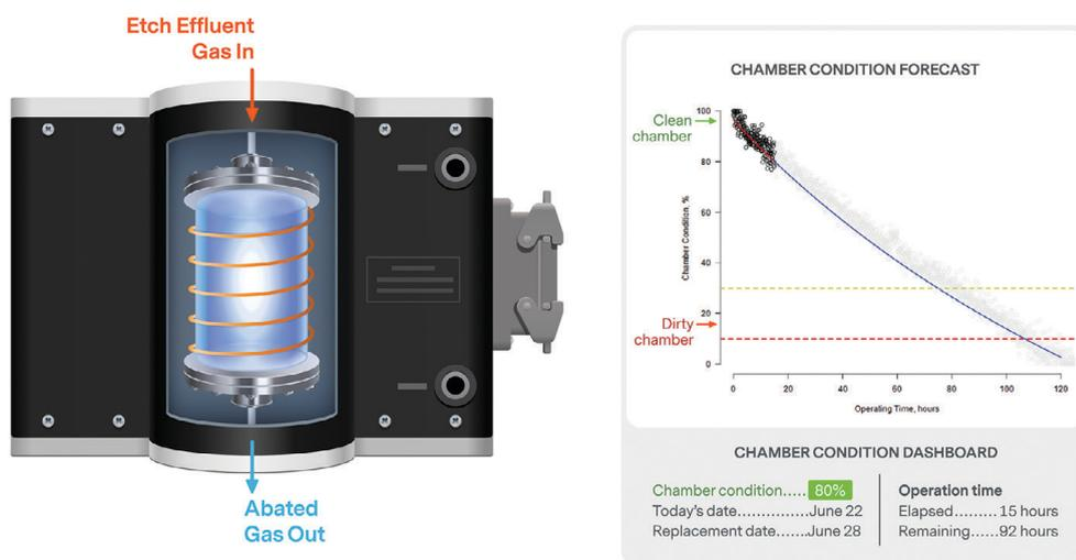
**Figure 10.** Abatement chamber (left) with chamber condition dashboard (right) showing figure-of-merit (chamber condition 0-100%) on vertical axis, and operation time on horizontal axis.
