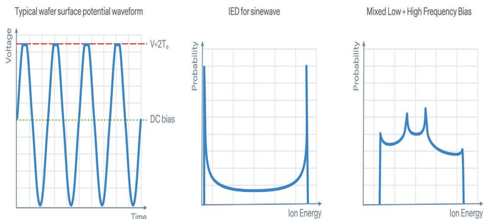
**Figure 6.** Oscillating voltage (left) from RF biasing translates, by virtue of its probability function, to (middle) bimodal ion energy distributions; mixing multiple frequencies leads to additional modes and more complex energy distribution functions (right).
