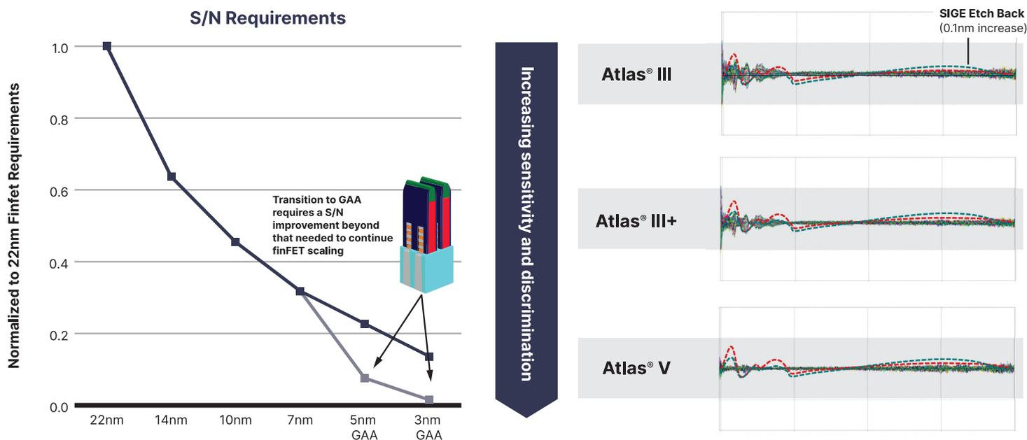
**Figure 4.** (Left) GAA transistors offer better performance than finFETs but are more complex and require a significant improvement in S/N of OCD measurement systems. The spectra (right) the steady improvement in S/N over three generations of OCD metrology systems.
