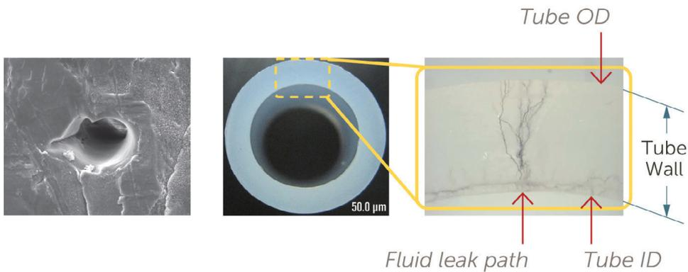
**Figure 2.** Left: Magnification of pinhole in a valve diaphragm. Center/right: Example of electrical discharge through a standard PFA tubing wall (0.062" diameter wall thickness).
