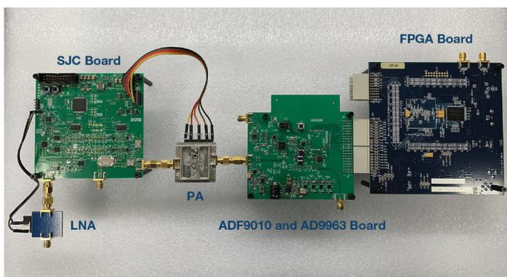
**Figure 5.** Test setup photo.
