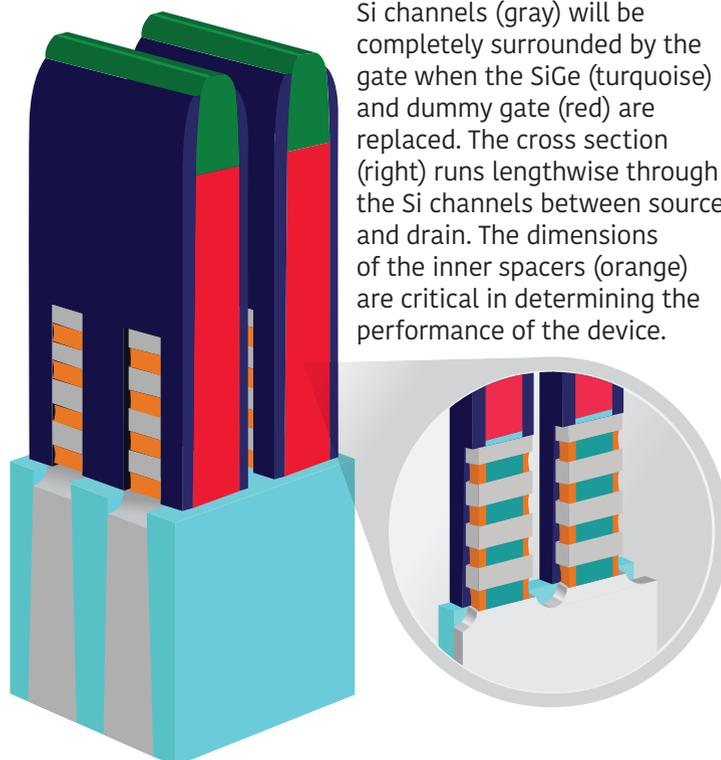
**Figure 3.** GAA transistor - the Si channels (gray) will be completely surrounded by the gate when the SiGe (turquoise) and dummy gate (red) are replaced. The cross section (right) runs lengthwise through the Si channels between source and drain. The dimensions of the inner spacers (orange) are critical in determining the performance of the device.
