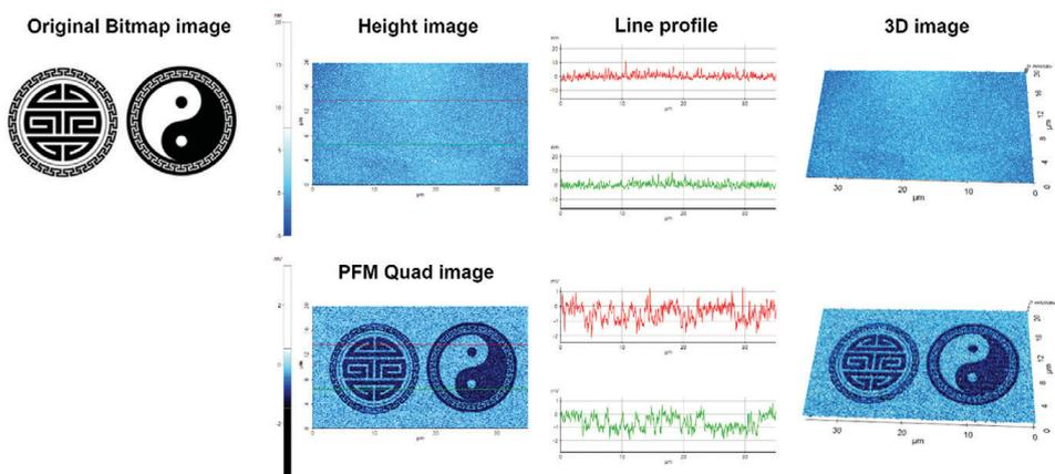
**Figure 5.** Original bitmap images used as templates (left), AFM height and PFM quad images after ferroelectric switching in AFM nanolithography bias mode, line profile analysis (center) and the corresponding 3D images (right). The nanopattern on PZT was generated by ferroelectric domain switching.
