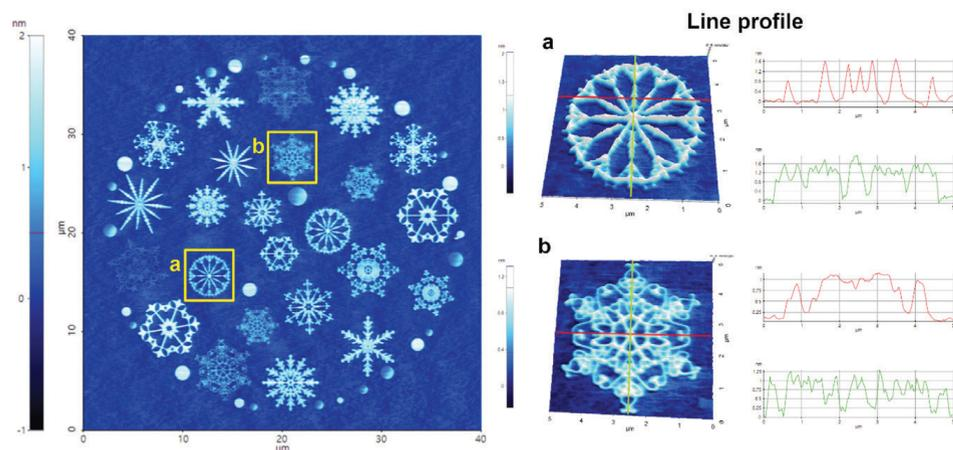
**Figure 4.** AFM height images after nanolithography and line profile analysis on two of the constituent structures. AFM line profiles in a and b show the ~1 nm height of the oxide layer from the substrate.
