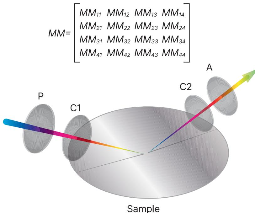
**Figure 2.** An ellipsometer compares incident polarized light and reflected polarized light to determine structural and material properties. With two compensators, it can acquire all 16 elements of the Mueller matrix that completely describes the reflection.
