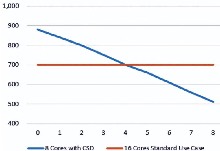
Figure 2. Deployment of SSDs versus CSDs using the TERASORT benchmark highlights where performance is accelerated with additional CSDs. Source: Mentor, a Siemens Business
