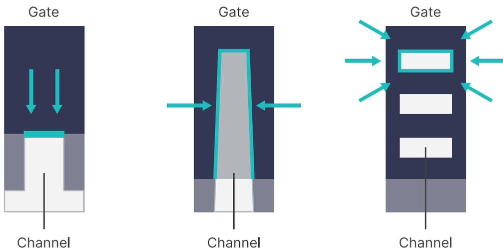
Figure 1. Planar, fin and gate-all-around field effect transistor architectures [1].
