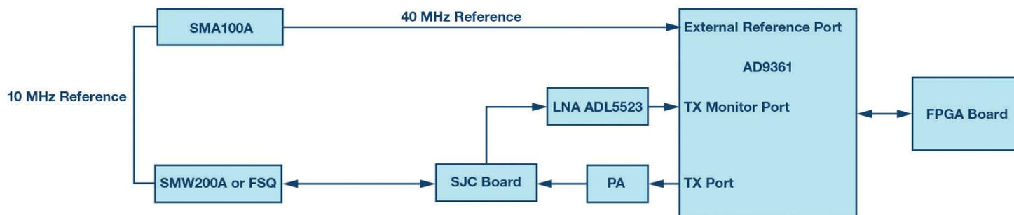
**Figure 9.** Test setup block diagram.
