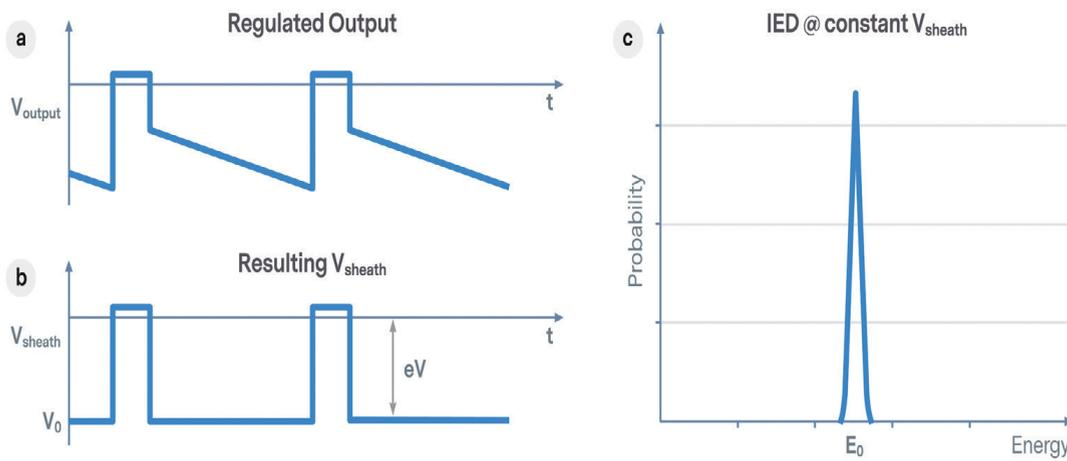
**Figure 7.** In asymmetric biasing, the Ion Energy Distribution can be directly controlled by regulation of the sheath voltage. Controlling the magnitudes and slopes of the output waveform (a) provides user control of sheath voltage (b). Narrow Ion Energy Distribution (c) is achieved when the sheath voltage is regulated to constant value.
