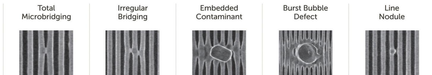
Figure 1. Photolithography wafer defect type examples.
