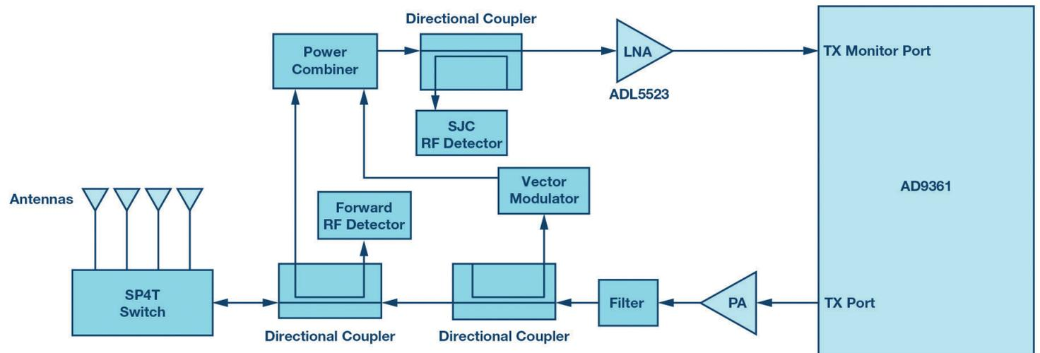
**Figure 7.** Received receiver data FFT plot and decoded data. **Figure 8.** A UHF RFID reader RF front end using an AD9361 block diagram.
