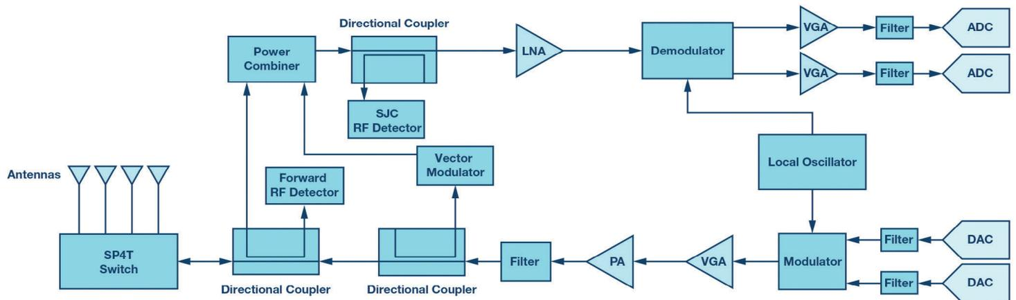
**Figure 3.** UHF RFID reader RF front-end block diagram.
