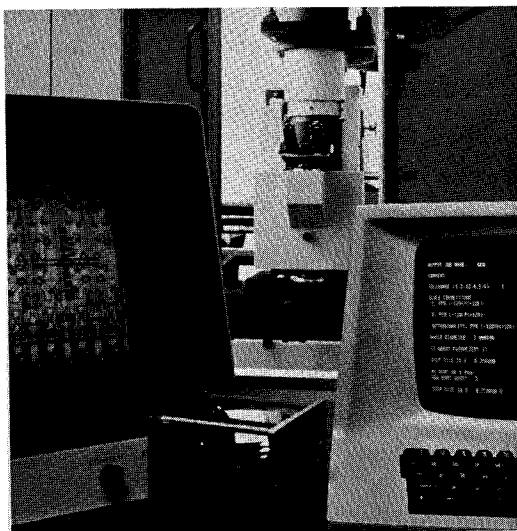
Fig. 16—Alignment microscope utilizing "off-axis" alignment.
