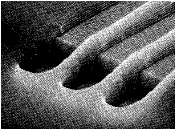
Fig. 2—Positive resist (AZ 1370, 10,000Å) SiO 2 -1 μm step; (1.0 μm geometry).
